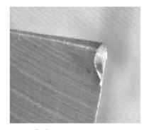
Figure 5: Severe Flank Wear on Tool
