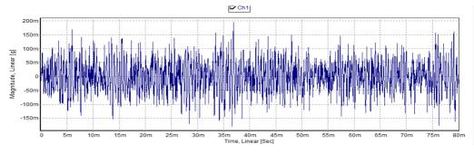
Figure 9: Amplitude-Time Spectrum of Medium Wear Condition (0.3 mm Flank Wear)
