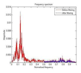
Figure 10: Filtering Signals above 5 Khz Using Filter
