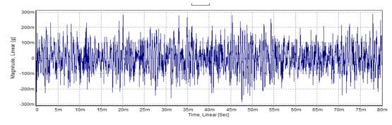
Figure 12: Amplitude-Time Spectrum of Severe Wear Condition (above 0.6 mm Flank Wear)
