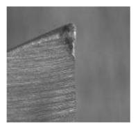
Figure 4: Medium Flank Wear on Tool
